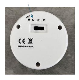
**R – Record**: The device is ready to record, hold down the button and speak clearly.
